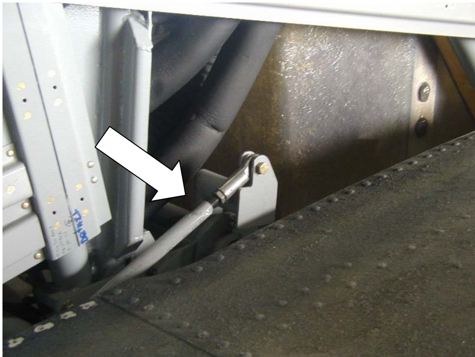
Figure 48-2: Inspection location for right end of torque shaft. Left opposite.
